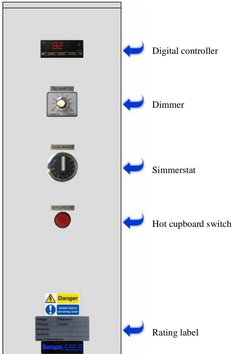
**Digital controller** - This is used to display the temperature inside the Hot Cupboard. The digital controller will only illuminate when the unit is switched on by pressing the hot cupboard switch.
